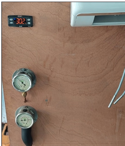
Figure 6. Temperature sensor calibration check in ambient air
