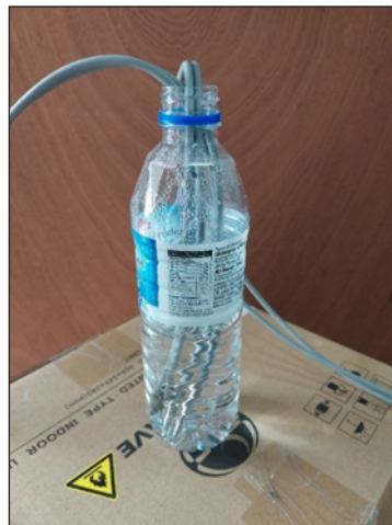
Figure 7. Temperature sensor calibration check in water medium
